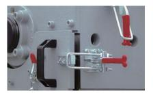
The Virtus Quick Snap System allows the lower front plate section to be easily removed for granulator cleaning. The lower front plate section is held in position by two sturdy lever clamps.
