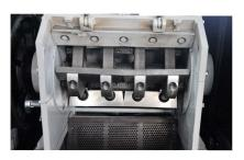
The cutting chamber sits in a soundproofed enclosure to ensure quiet inline operation. The rotor and screen area are easily accessible for cleaning and maintenance without the need for additional tools.
