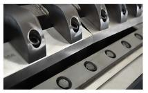
The H granulators are available with different rotor options to fit different applications, all rotors feature the V-cut technology creating a high quality regrind.
