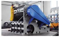
The granulators can be tailored to fit various applications, for example with oversized suction troughs in order to achieve a very high output.
