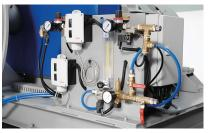
The material temperature is monitored in the process, and an automated cooling system will ensure the temperature is kept at a defined level.
