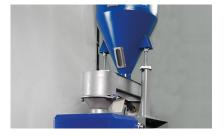
The material is fed into the Pulverizer by a vibrating dosing channel, and the feeding rate is automatically adjusted based on the motors amperage and material temperature.
