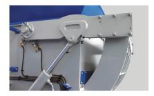
The G series shredders benefit from sturdy ram construction incorporating heavy duty guide bearings and universal couplings for reliable operation.
