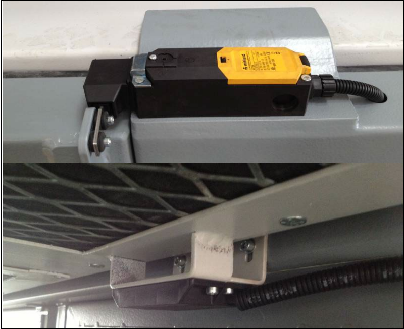
Illustration: Safety device for housing flap and hopper
