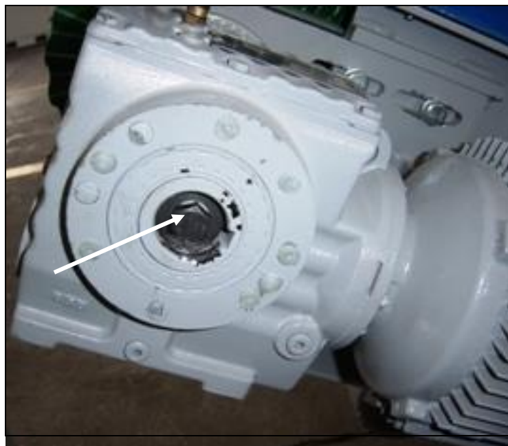
Illustration: Fixing screw on the shaft
