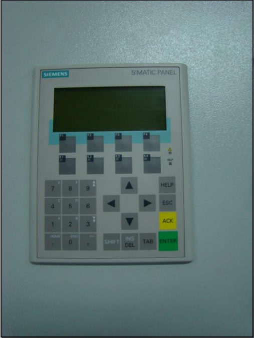
Illustration: HMI operator panel
