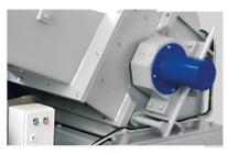
The heavy duty bearings are separated from the cutting chamber to avoid lubricants entering the cutting chamber, and bearing failure due to material contamination.
