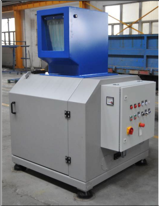
Illustration: Granulator type C with soundproof box and soundproof hopper.
