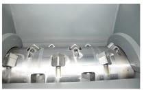
All Virtus shredders are equipped with our E-style flat rotor. The knives are fixed in special knife holders fitted in machined pockets.
