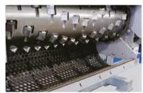
All **Virtus** shredders are equipped with a large diameter flat rotor. The knives are fixed in special knife holders fitted in machined pockets. Optional weld on hard facing is available for abrasive applications.
