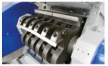
The specially angled rotor automatically pulls the fed pipes or profiles into the cutting chamber, this design also regulates the amount of material.
