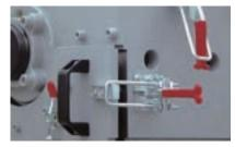
The Virtus Quick Snap System allows the lower front plate section to be easily removed for granulator cleaning. The lower front plate section is held in position by two sturdy lever clamps.
