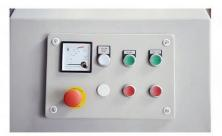
To minimize the needed floor space and make the machine easy to move, machine controls and electrical cabinet are integrated into the machines soundproof housing.
