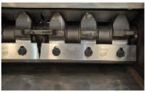
The granulator part uses a sturdy F+ rotor to ensure a good ingestion of the material flow while still being able to handle thicker and heavier particles.
