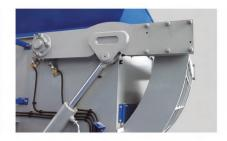
The G series shredders benefit from sturdy ram construction incorporating heavy duty guide bearings and universal couplings for reliable operation.
