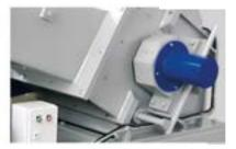
The heavy duty bearings are separated from the cutting chamber to avoid lubricants entering the cutting chamber, and bearing failure due to material contamination.
