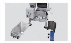
Due to the Quick snap fasteners used on the A Series 30, the machines can be opened for cleaning and maintenance quickly without the need for special tools.
