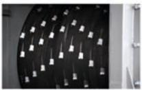
The P shredders use very large diameter flat E-style rotors. The knives are fixed in special knife holders fitted in machined pockets.
