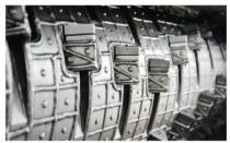
The T shredders are equipped with large diameter flat rotors with weld on hard facing. The knives are fixed in special knife holders fitted in machined pockets.
