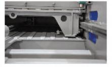
The SG system uses a sturdy, roller guided drawer type ram to feed the material into the shredder. Segmented cutting chamber and ram allow trouble free processing of thin materials.
