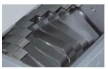
Staggered rotor blades create an individual blade cut thus increasing the cutting torque. All of the machines in this series are therefore suitable for grinding more solid materials and thicker walled sprues.
